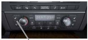
Seat heating/ventilation adjustment buttons
