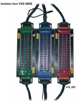
For diagnostics on new-generation control modules with 198-pin terminals (UDS control module). The illustration shows a prototype.
