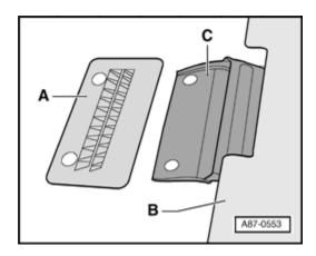
\* Heater element is installed only on vehicles with Rear A/C Control Head (Climatronic) E265 in vent - **C** - (optional equipment).
