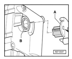
Attach connecting element - A - onto actuator shaft.
