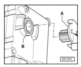
Attach cam disk - A - to actuator shaft.
