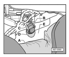
The following illustrations show the evaporator drain for the right side of the vehicle.
