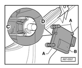
Remove and install Right Rear Warm/Cold Flap Air Outlet Motor V221 - B - in the same manner as described for Left Rear Warm/Cold Flap Air Outlet Motor V220 ⇒ Left Rear Flap Air Outlet Motor .
