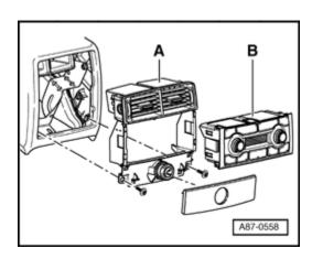
Remove vents from rear center console - A - . Without Extension ⇒ Body Interior -Repair Group 68 With Extension ⇒ Body Interior - Repair Group 68
