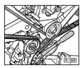
The toothed belt tension adjustment is done by turning the tensioning roller with 8 mm hex-key wrench.
