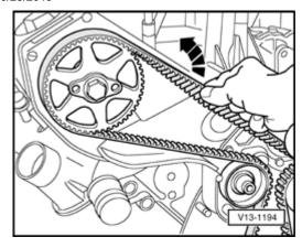
Check belt tension by gripping belt halfway between camshaft sprocket and coolant pump.
