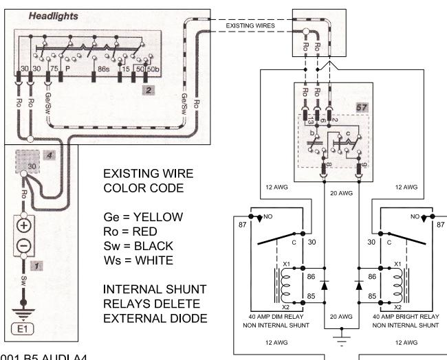
1996 - 2001 B5 AUDI A4 HEADLIGHT POWER SWITCH ADDED RELAYS MODIFICATION.
