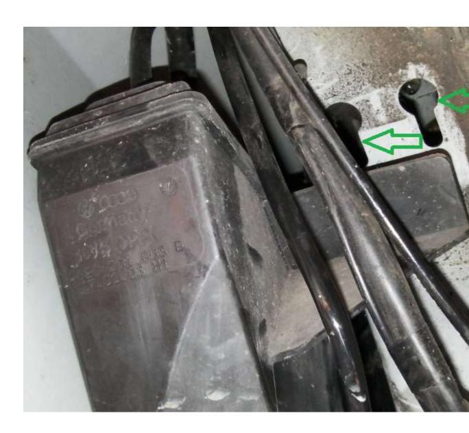
5. Remove the soft black filler to reveal the bolt head on the hinge. The first pic below shows the lower hinge bolt, and the  $2^{nd}$  pic shows the filler removed.
