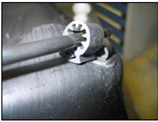
Close rubber clip and allow ventilation line to rest on fuel tank (as shown); proceed to Section C
