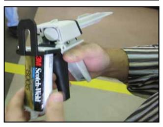
Insert adhesive cartridge (Z3MDP8005) in the VAS 5155 applicator gun and remove cap
