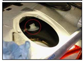
← Clean rollover valve carefully with cleaning fluid (D 009 401 04) to ensure valve is free of dust and grease
