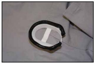
Remove mold from rollover valve, then place butyl cord around mold
