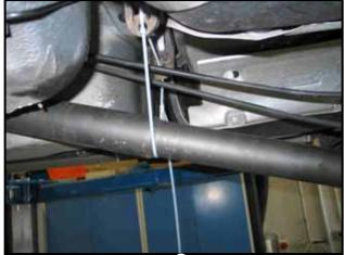
□ Detach driveshaft from rear final drive, lower it slightly (max. permissible angle 15°) and tie wrap to exhaust system brackets
