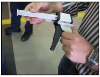
Assemble VAS 5155 applicator gun by sliding the VAS 5155/3 (10:1) plunger into applicator gun
