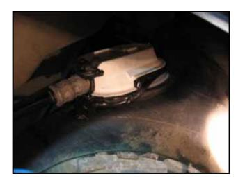
If black mold (shown white in picture) and 3M<sup>™</sup> adhesive are present, <u>no further work is required;</u> otherwise, proceed to Section B
