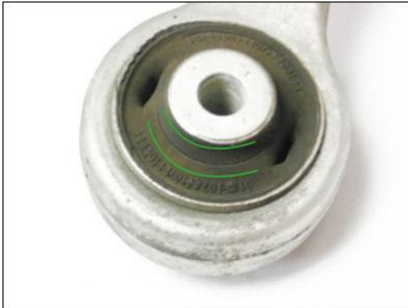
Figure 5. A bushing with a hairline crack. This is an acceptable amount of wear.
