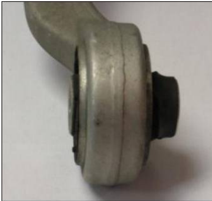
Figure 3. A bushing with a displaced insert.
