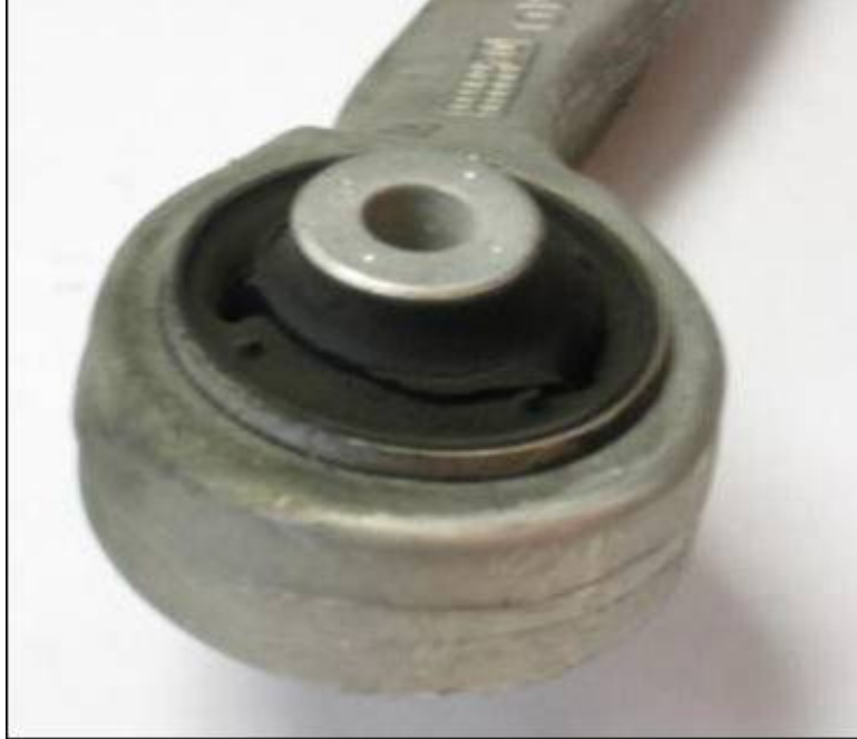
Figure 2. A bushing with cracked rubber.
