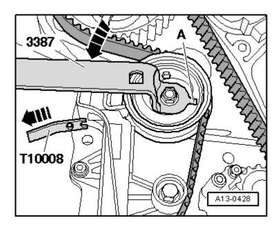
Turn eccentric pulley counterclockwise using pin wrench 3387 (tab - **A** - of eccentric pulley must not be bent), until die T10008 can be pulled free of stress.
