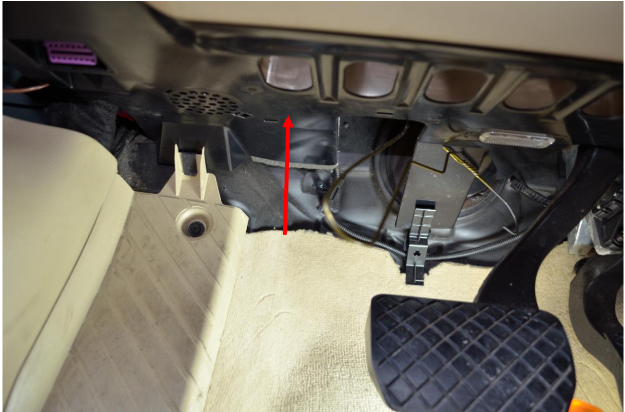
Figure 3 - Pass through hole above here
