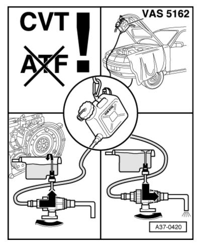
Attach filled reservoir of ATF charging device for CVT gearboxes -VAS 5162- at the highest possible point on the vehicle.
