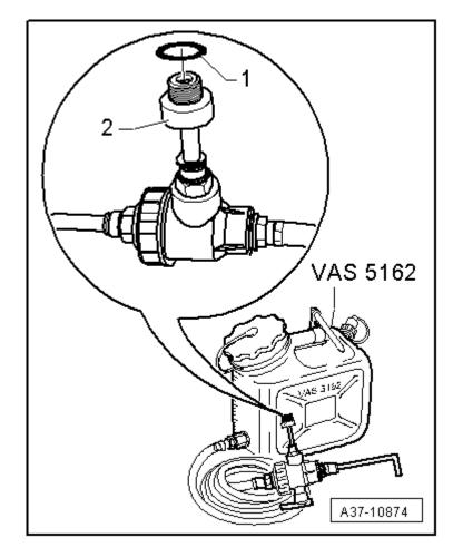
With O-ring removed, screw connection of ATF charging device for CVT gearboxes -VAS 5162- hand-tight all the way into threaded hole for ATF inspection plug.
