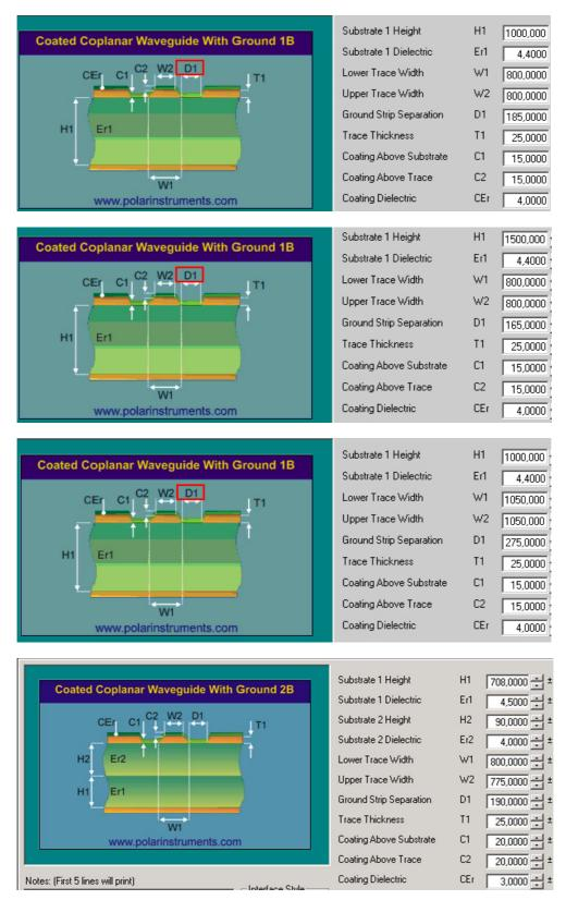
Figure 6: Micro-Stripline line arrangement samples
