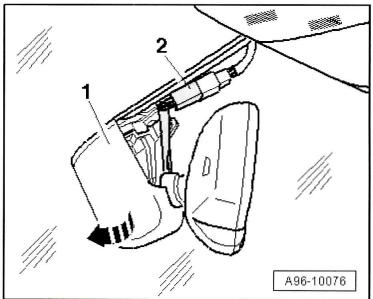
Carefully disengage the tabs -arrowsand remove the front cover -1downward out of the guide rods on the rearview mirror base -2-.
