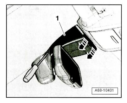
Unclip cover -1- at the mirror base using a screwdriver and remove it.
