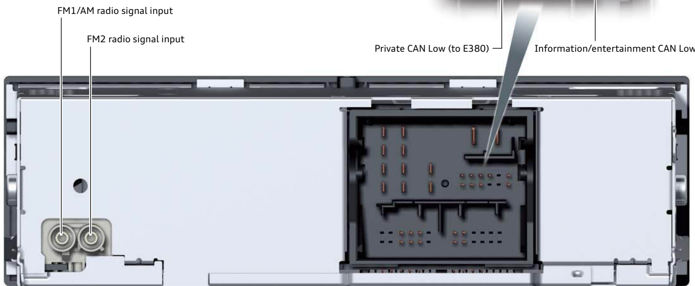
Rear panel of J794 for Entry MIB
