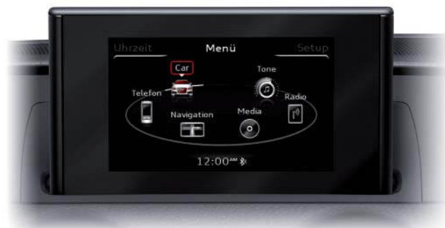
MMI screen for Standard MIB with active navigation system on Audi A3 '13
