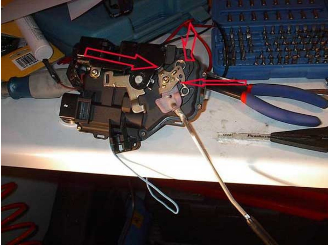
You're done! Here you'll see where the springs are connected.
