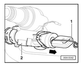
Insert steel wire or pin (approx. 1.5 mm Ø) -1-, as illustrated up to stop while pulling lock cylinder with induction coil out of steering column housing -2- in direction of arrow.
