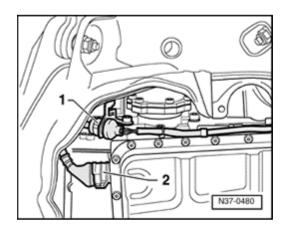
Disconnect electrical connector - 1 - on Multi-Function Transmission Range (TR) Switch F125.
