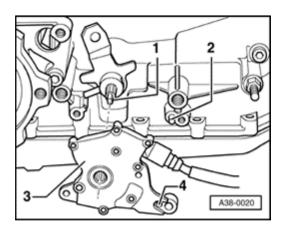
Connect Multi-Function Transmission Range (TR) Switch F125 to shift rod. Flat part at splines in switch - 3 - must align with flat part of shift rod - 1 - .
