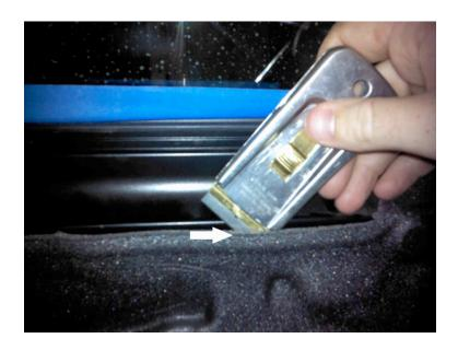
After removing the motor, you can now remove the insulation. It has thick glue on the reverse that can be cut through using a razor blade. Remove the insulation and place to one side.
