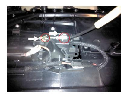
After removing the door panel, support it, and remove the door handle cable by pulling the white clip out and unhooking the cable.
