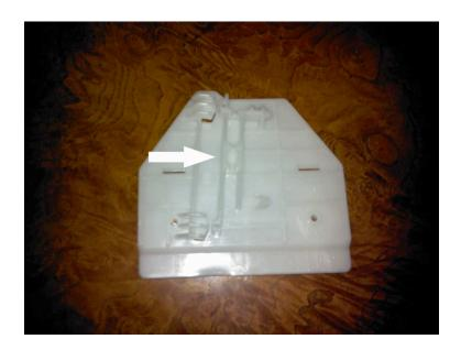
Note the location of the bead holder on the new regulator clip. On the damaged part, this is the spot that usually breaks.
