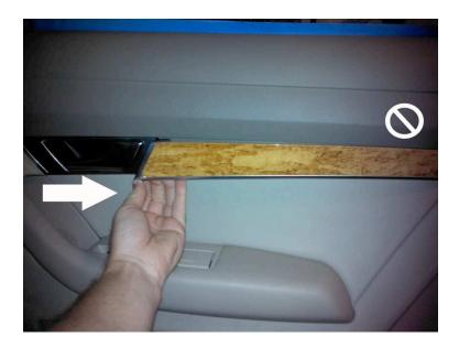
Begin by removing the wood/aluminum trim. Simply put your hand under the left side of the trim, and pull towards you. Make sure you start on the left side of the trim, if you pull the right, it will break the L shaped clip on the rear of the trim.
