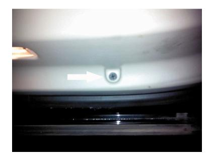
Remove the last Philips head screw on the bottom of the door panel.
