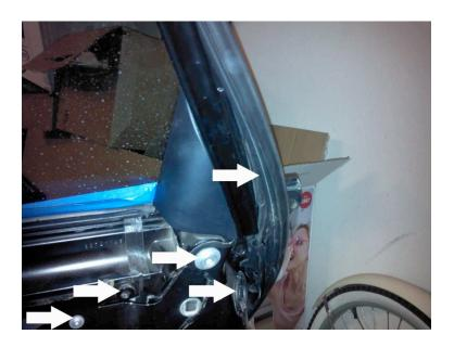
Next, on the outside of the door, pull the door seal away from the window frame. You only need to remove it from the top part of the door. Also remove the three Torx screws show in the picture above. On the end of the door there is a plastic cap (bottom arrow), remove this cap and inside you'll find a fourth T-40 Torx screw to remove.
