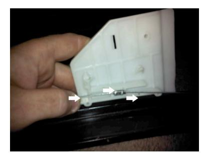
Insert the new regulator clip by aligning the clip to the rail, place the bead in the clip, holding the cable with your thumb. Twist down and snap the regulator clip into position, check that the gears turn when you slide the window up and down. That's it!
