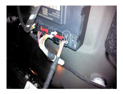
Next, disconnect the door wiring harness. Pull the red clip out, it only moves ¼ inch. Then press the exposed black tag down, and remove the connector. BE CAREFUL it's easy to break it. Remove the door panel and place to one side.
