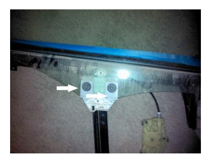
Now remove the two Torx screws holding the regulator clip to the window, it helps if the window is fully closed at this point.
