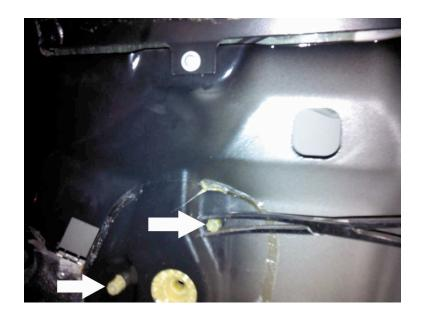
Using some long nosed pliers, squeeze the protruding screw mounts on the window regulator. Push them through the door.
