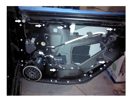
Remove all the Torx screws where indicated, there are 6 of them. The ones on the top of the door hold the window frame in. the ones on the bottom hold the regulator to the door.
