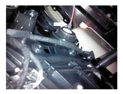
Next, disconnect the loudspeaker wire, the clip is on the bottom of the connector, just squeeze and remove.
