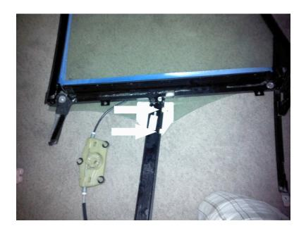
Place the window frame on a soft surface, like some carpet, and note the way that the window regulator clip attaches to the slide. It's a good idea to add some silicone grease here if it has gone dry.
