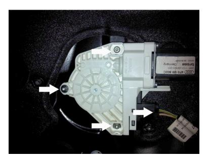
Next, remove the window motor, there are three Torx type screws to remove and one electrical connector. Place the motor to one side.
