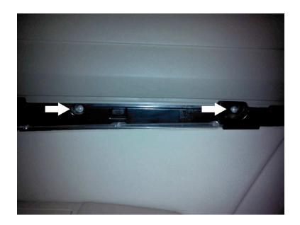
After removing the trim, two Philips head screws are exposed, remove them both.
