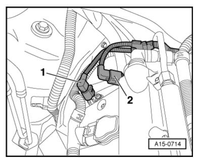
Disconnect electrical harness connectors -1and -2- at Camshaft Position (CMP) Sensor -G163- and Camshaft Position (CMP) Sensor 3 -G301-.
