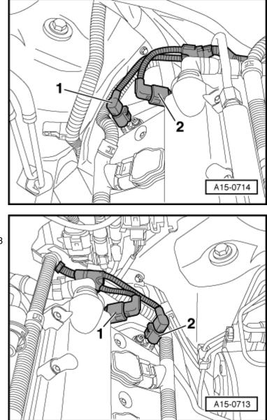
Disconnect electrical harness connectors -1and -2- at Camshaft Position (CMP) Sensor -G163- and Camshaft Position (CMP) Sensor 3 -G301-.
