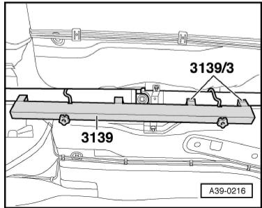
Remove securing nuts -arrows- for intermediate bearing.
