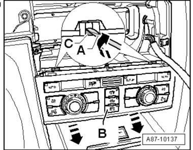
Reach beneath the operating and display unit, Climatronic control unit -J255--A- and pull it carefully out of the centre console (operating and display unit with "pearl grey metallic" trim).
