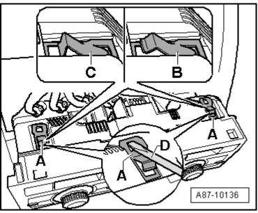
Nero), the operating and display unit can only be removed after taking out the centre dash panel vent  $\rightarrow$  Rep. Gr.68. To enable the clips -C- to be unfastened, a slot -Dhas been provided in the dash panel centre section in the area of the upper support brackets for each of the clips.
