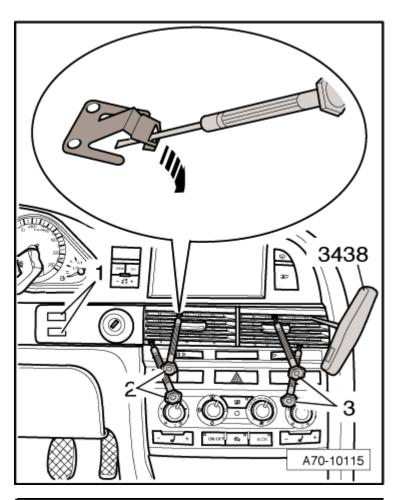
Press the hazard warning light switch -E3-item 1- out of air vent trim -arrow-.
