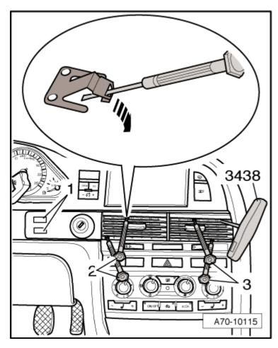
If is is not possible to pull out dash panel vent as described, perform the following procedure:
