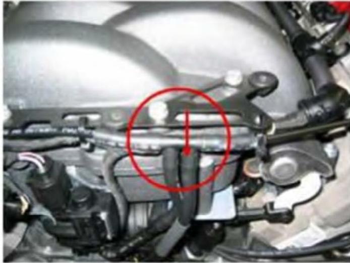
Figure 5. The lower left hose on the double T pipe.
