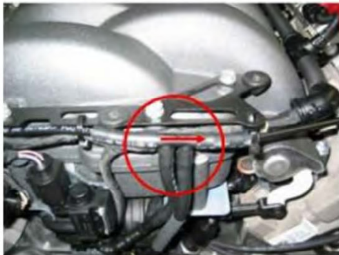
Figure 2. The upper left hose on the double T pipe.
