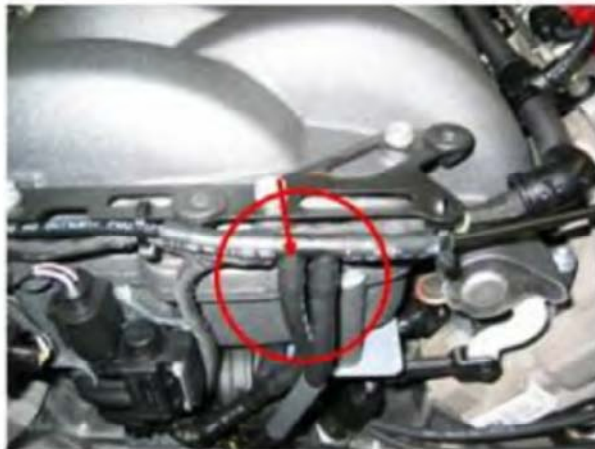
Figure 1. The lower right hose on the double T piece.
