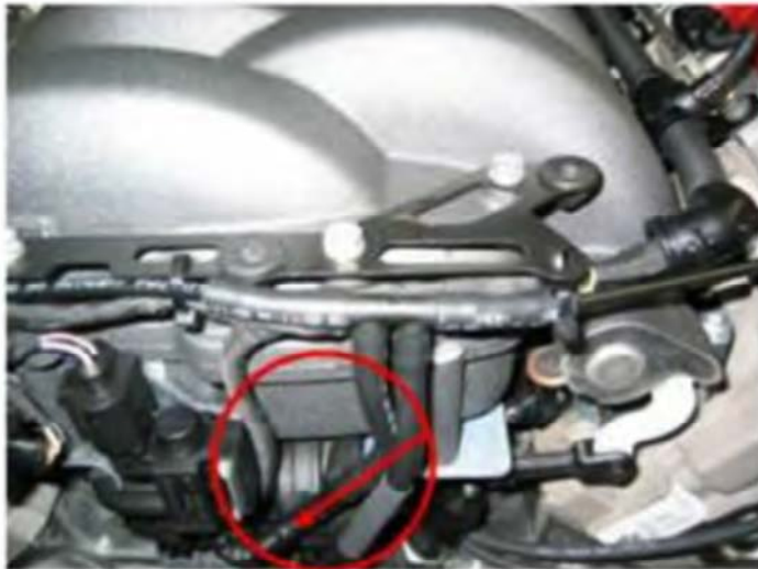
Figure 3. The lower T pipe of the lower hose.
