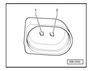
Using a Multimeter , check the resistance between terminals 1 and 2 of the Evaporative Emission (EVAP) Canister Purge Regulator Valve N80 .
