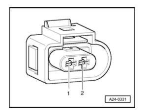
Using a Multimeter , check the Evaporative Emission (EVAP) Canister Purge Regulator Valve N80 electrical connector terminal 2 to the Engine Control Module (ECM) J623 electrical connector T94a terminal 9 for an open circuit.
