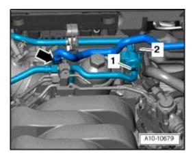
Disconnect the Evaporative Emission (EVAP) Canister Purge Regulator Valve N80 electrical harness connector - 2 - .
