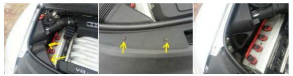
Remove the 2 screws holding the air intake duct in place using a Phillip screwdriver, and remove the duct assembly (note: the intake duct is a two piece assembly).
