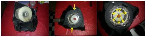
Remove two screws that hold the air filter to the housing (see arrows in center picture) and pull the filter from the housing. Remove large gasket and discard.
