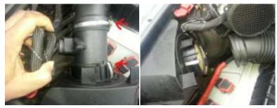
Loosen the hose clamp (using flat head screwdriver), and disconnect the 2 clips on the air filter housing to and remove the Mass Airflow Sensor (MAF) assembly in order to have room to maneuver the air filter assembly for removal.
