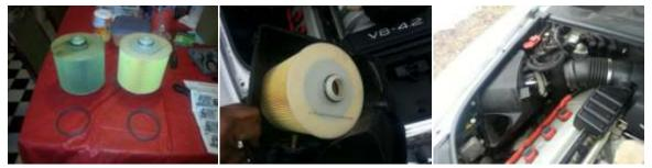
Coat both large and small gasket with light grease (included with replacement air filter). Small gasket should already be on small end of filter that seals the filter to the air filter housing base. The larger gasket is what seals the MAF housing to the Air Filter housing. Reverse this procedure to attach air filter to housing , and to reattach filter assembly to the car.
