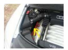
The Engine Air filter is located on the right side just in front of the firewall.
