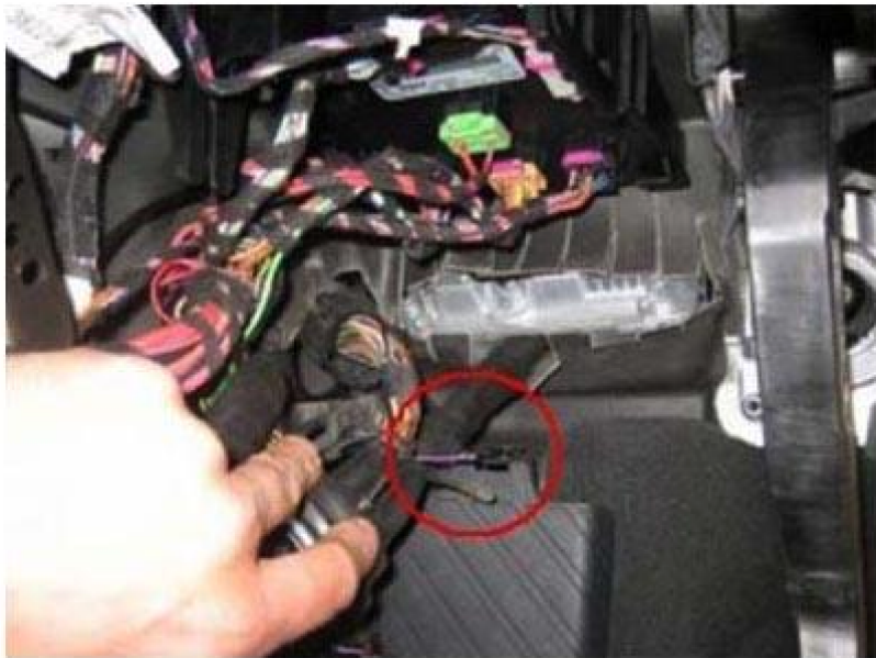
Fig. 1: Wire Harness In Driver Footwell Area
