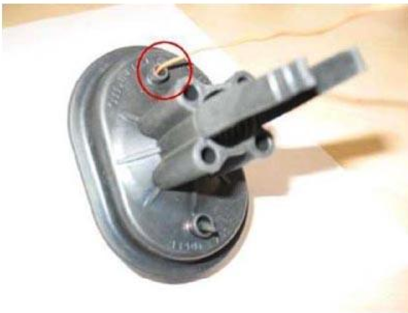
Fig. 4: Seal Off Access Hole In Grommet With Butyl Sealant
