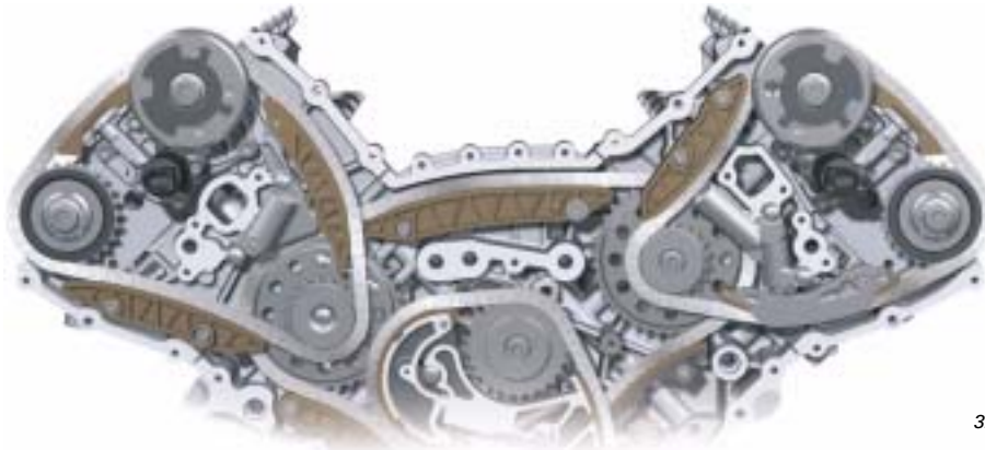
Camshaft adjuster, intake camshaft cylinder bank 1
