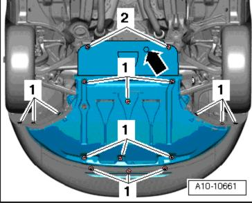
Remove the bolts-1-and-2-for the left and right stabilizerm ounts and lower the stabilizerbarslightly.
