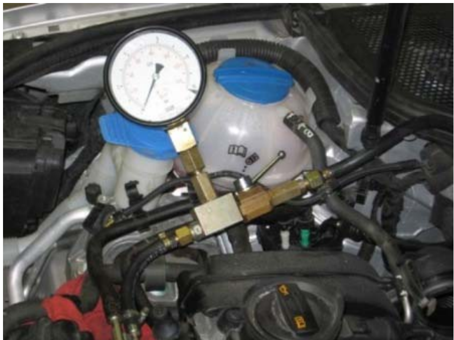
Figure 1. VAG 1318 gauge installed on an A3 2.0L TFSI vehicle.
