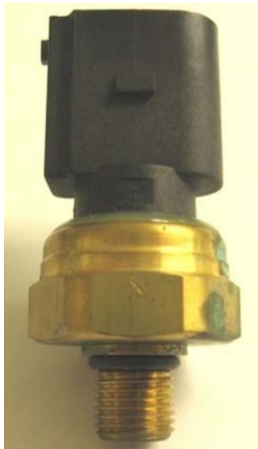
Figure 2. Fuel pressure sensor 06E 906 051 J.
