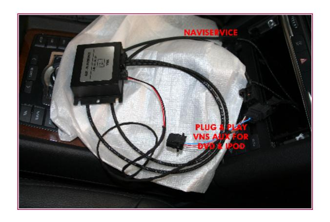
9.CONNECT POWER SUPPLY VNS AUX BY MEANS OF PLUG&PLAY
