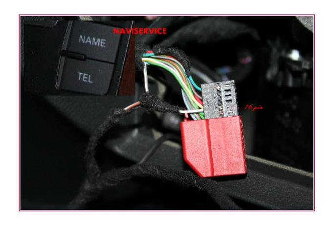
3. TO 16PIN PLEASE CONNECT WIRE FROM CABLE HARNESSES OF MULTIMEDIA ADAPTER. IT WILL ENABLE YOU TO CONTROL/SWITCH OVER AV1/AV2/AV3/RGB AND SWITCH OF MULTIMEDIA ADAPTER BY BUTTON "NAME".
