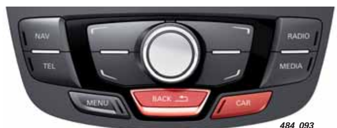
Button combinations for the Engineering menu
