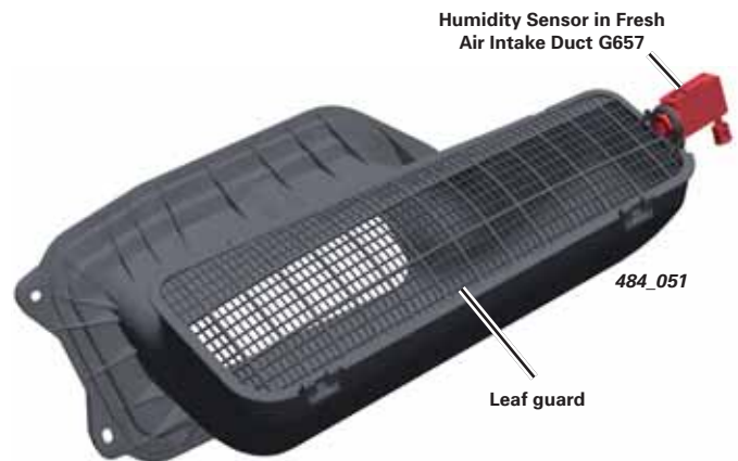
Humidity Sensor in Fresh Air Intake Duct G657 in the three-zone climate control system
