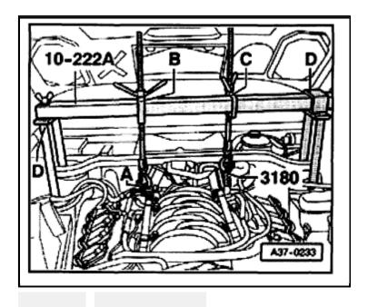
Install 10 - 222A engine support bridge with 10 - 222A/4 adapter for engine support -arrow D- to bolts of suspension strut connection.
