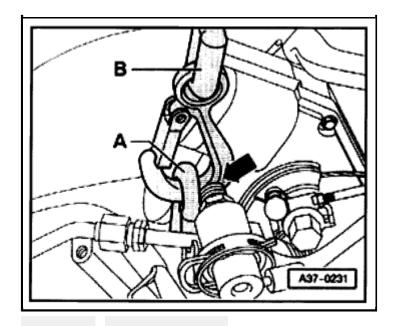
• Be sure when lifting and lowering engine that hook -B- or auxiliary hook -A- do not come in contact with fuel pressure regulator -arrow-.
