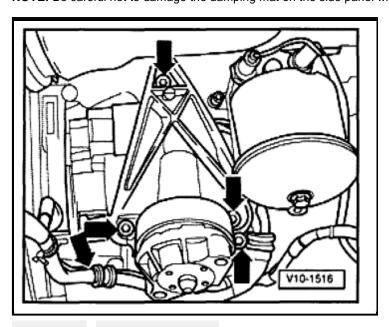
• Remove right engine mount and wiring clamps -arrows-. Position engine mount on engine/transmission carrier.
