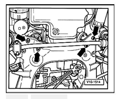
• Remove lower bolts -arrows- at engine mounts.
