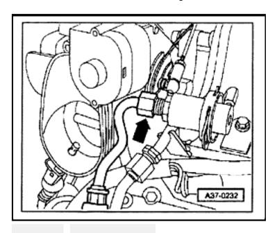
• Disconnect fuel line from fuel pressure regulator -arrow-.
