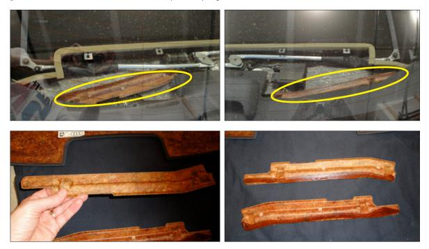
It seemed that over time the glue that held the two objects in place failed and left the two objects laying on the metal rear shelf. When ever I went over a bump or rough surface the two objects would mover around causing the rattle. Once the two objects were removed; the rattle was gone.
