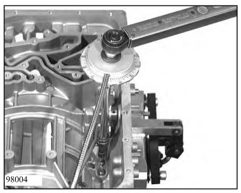
Align the detent spring's roller on the center of the detent disc, and screw it tight with helping tool 5w04 000 583 in this position.
