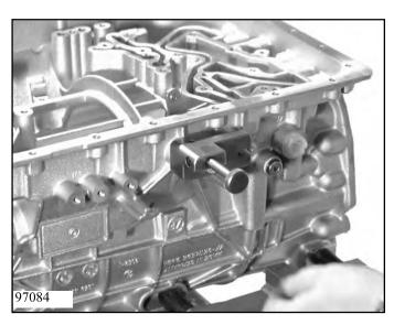
Place position gauge 5p01 002 839 on the selector shaft, turn the position gauge so that the locating pin in the transmission housing enters the cutout in the position gauge and eliminate any play by turning the knurled screw.
