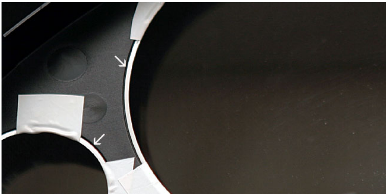
The arrows indicate the rim where the glue goes.
