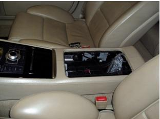
11. Fit the tray, place the rubber seal around bracket and place the armrest in its place. Tighten the 3 T45 screws and finally fit the cover.
