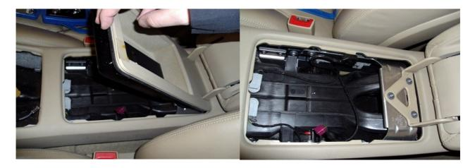
7. Remove the screw holding the front air duct and the 2 holding the fron ACpanel. Unplug conectors and remove panel. Behind it are 2 more screws holding the console so remove those as well.
