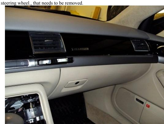
Then take away the fuse box covers on each side of the instrument panel. Remove 2 screws on each side. Now there's only one more screw at the bottom right of the knee panel before you can lower it down enough to get to the last screw holding the console on left side. It's located fairly low down.
