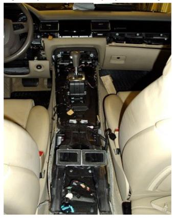
When console's gone, remove the front air ducts and transfer them to the new one.
