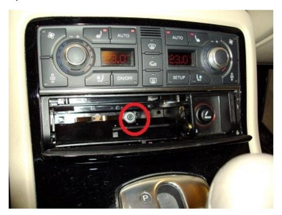
4. Grab the trim in any of the lower corners and carefully lift it up, work your way backwards until it comes loose. Unplug the 3 electrical connectors
