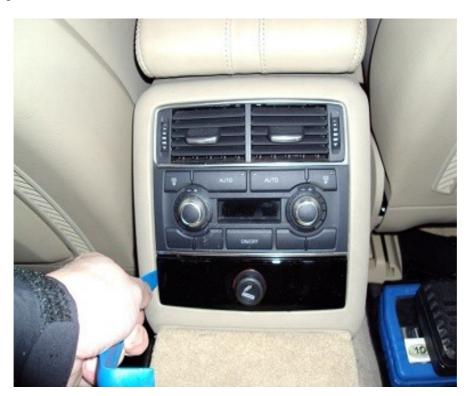
2. Remove the screws (1/side) holding the rear air ducts. Then remove the brackets (3 screws/side) and remove the 2 M8 nuts holding the console to the floor
