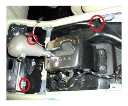
8. In order to get to the last 2 screws you need to drop the glove compartment and the knee panel. Start by pushing out the coin tray, grab the front cover of it and push it to the left so it comes off. Then pop out the grey plastic trim toward the passenger door and work your way toward the steering wheel. Remove the small grey trim toward the drivers door as well. With the trims gone you can see 2 T20 screws holding the knee panel, one on each side of the
