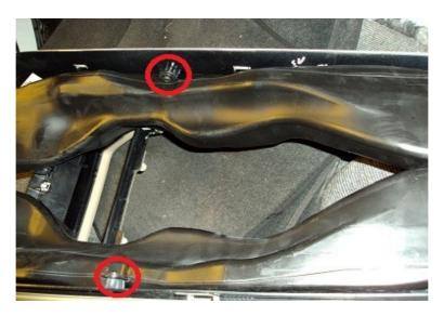
10. Before fitting the new console you need to fit the bracket for the new armrest. Bolts are already there so just remove the cut outs in the foam (see arrow), put the bracket in place and take 4 nuts to attach it. Once in place you can start refitting everything. Nothing strange about this, only make sure the carpet gets in the correct slot
