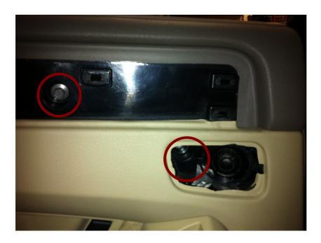
Finally you have one 8mm bolt in the storage compartment. Do NOT fold out the tray as you may drop the bolt behind it.
