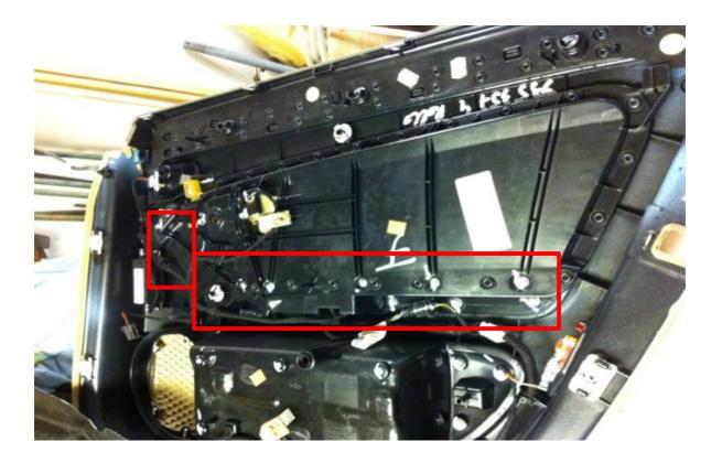
4. Now you can remove the complete handle. I want to replace the fake leather part with a real leather one so to separate the handle a T20 screw close to the window switch needs to be removed, then just pick the handle apart, fit the new one and reverse the above.
