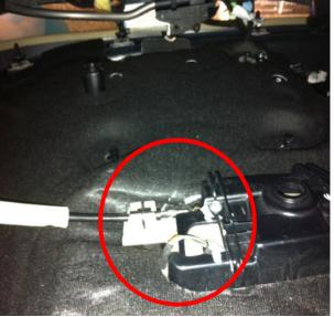
3. With the panel off you need to remove the liner, which sits with some special washers that just unscrew
