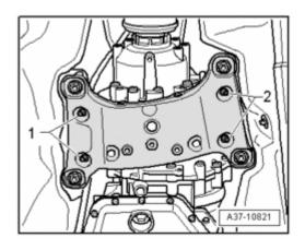
Remove left - 1 - and right - 2 - transmission bolts on tunnel cross member.
