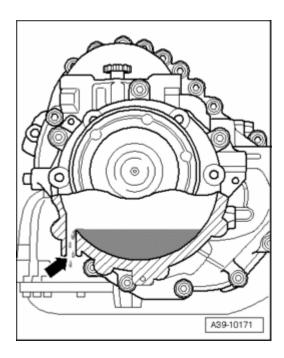
Slowly add axle oil into transfer case housing using a hose and a sprayer or pump in oil filler hole - arrow - .
