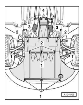
= Remove both rear noise insulation by loosening bolts - 2 - , - 3 - and - 4 - .
