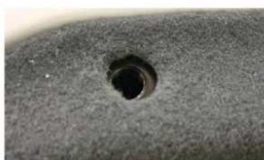
Figure 3. Bump stop unscrewed from trunk lid.
