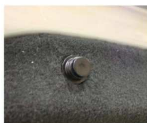
Figure 2. Rubber cover removed from bump stop.
