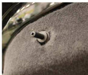
Figure 5. New spring-loaded pin installed.
