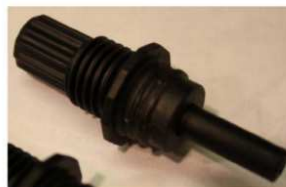
Figure 4. Rubber cover and spring-loaded pin removed from the new bump stop assembly.
