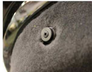
Figure 6. Depressed spring-loaded pin.
