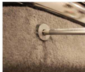
Figure 7. Philips screw driver used to eject pin. The rubber cover has been installed in this image.
