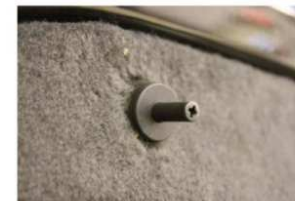
Figure 8. Spring-loaded bump stop installed.
