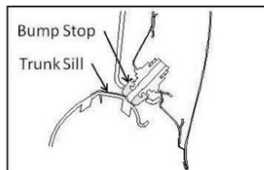
Figure 9. Side cross section of trunk lid closed and bump stop impacting the trunk loading sill.
