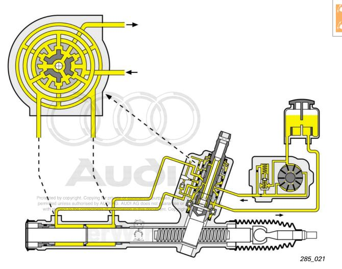
In the interests of clarity, the rotary slide is illustrated with 6 instead of 10 grooves.
