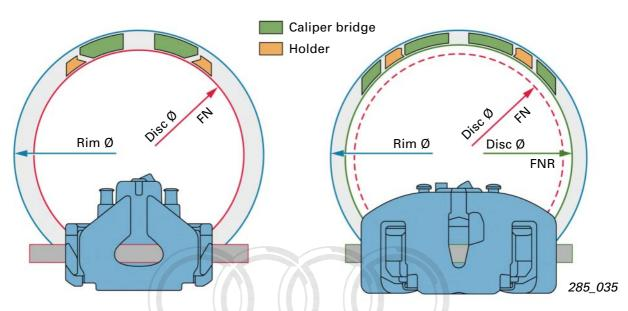
Comparison of technologies: FN and FNR disc brake in the same wheel
