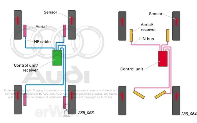
1st generation components and networking (Audi A8 up to `03)
