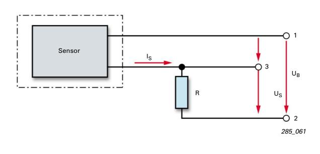
The output signal of the speed sensor is a PWM signal (PWM = pulse width modulation). The number of pulses in a specific time unit provides the
