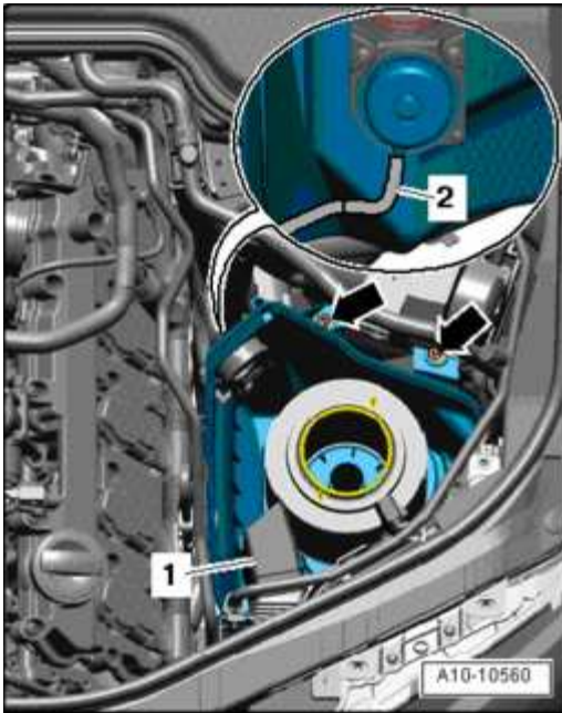
Fig. 762: Air Duct, Bolts, Air Filter Housing & Air Flap Vacuum Hose Courtesy of VOLKSWAGEN UNITED STATES, INC.
