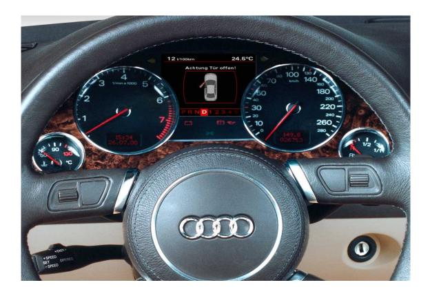
MMI functions can be controlled from the steeringwheel controls (above) or the center console (right). The MMI buttons shown control the radio, CD, navigation, and almost all vehicle settings - greatly minimizing the number of buttons necessary in the interior.
