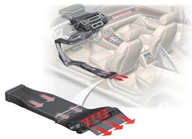
Attention to detail is an Audi hallmark. Notice how air is reheated just before the reaching the rear seat footwells. (shown to the left)
