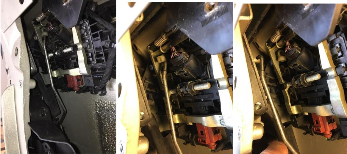
18. Once the latch rod is free, locate the electronic plug that connects to the handle for the keyless entry feature (I assume that's why you are replacing the handle in the first place). You can see it in the photos above. It is a good-sized D-plug, and a bit of a pain to disconnect. Pull up the outside handle up a little to make it easier to get the plug off. You can use a hook tool, or a small screwdriver like I did, to pry the catch on the D-plug so you can unplug it.
