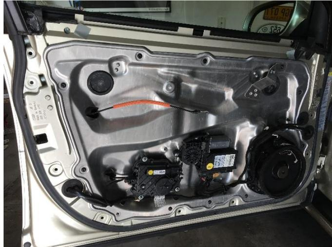
11. Door motor – three Torx 25 screws and three cables plugged in along the bottom. Once the screws are removed, pull the motor away from the panel and it'll be easy to unplug the cables.
