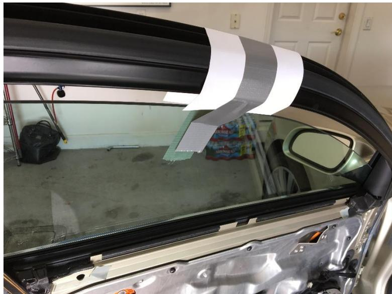
7. Unscrew the two bolts (Torx 30) holding the window. The duct tape should hold the window where it is and prevent it from sliding down.
