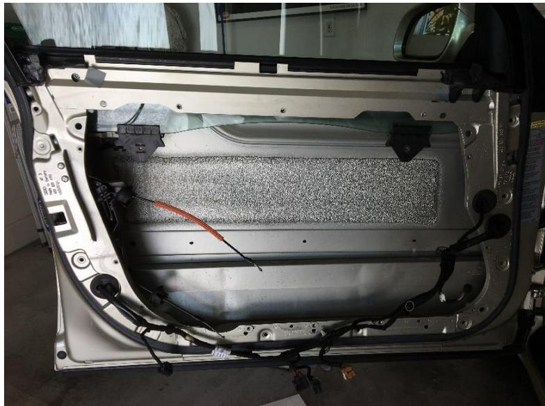
16. With the aluminum panel removed, you can see the door latch inside the door, and above that, the door handle. To make it easier to work on the handle, I lifted the window up as far as it would go (to the “window closed” position). Lift one side of the duct tape off the glass and pull the window up (with one hand on each side of the glass) until it is all the way up, and reattach the duct tape. Right, my window is now duct taped “fully up/closed.”
