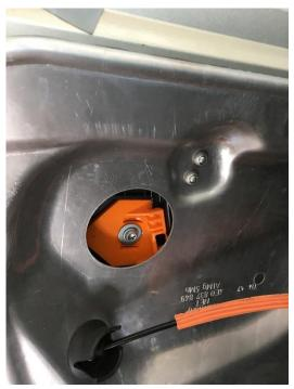
6. I used a piece of duct tape about 2 feet long, looped over the top of the door (with a piece of paper so the tape glue wouldn't mess up the door frame – see the picture) to secure the window in its lowered position. Then I affixed the tape to both sides of the window. Once those window bolts are removed, you don't want the window glass sliding down into the door – you want it to stay where it is.
