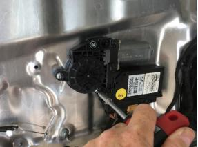
13. With the two motors removed, you can pull the cable harness along the bottom away from the aluminum door panel. The harness is held by snap-in tabs that will need to be pried out of their mounting holes. Unplug the door speaker connector as well. Right, motors are out and all wiring has been unplugged.
