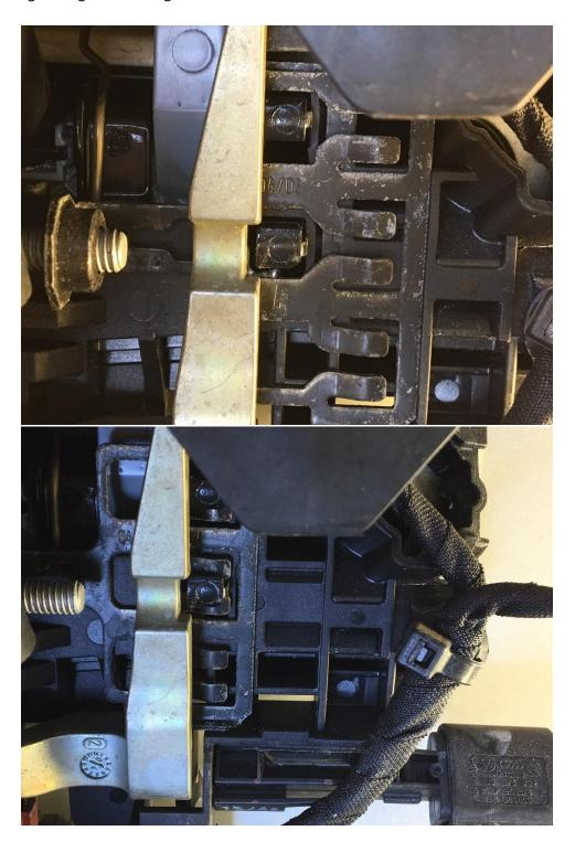
20. Once the grub screw is unthreaded all the way, hold the inside of the handle mechanism with one hand and the outside handle with the other, and work them apart until the outside handle comes off. It might take a little doing, and it's kind of a tight fit, so be patient to avoid damage to your door paint finish. Once it's out, clean the dirt and grime from the outside door surface.
