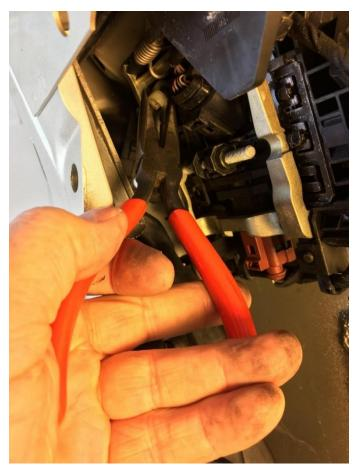
white plastic connector (and the handle). Below right, the latch has been removed from its mounting hole in the white plastic connector, and is free. Also note, the grub screw that removes the handle is visible in the middle of these photos.
