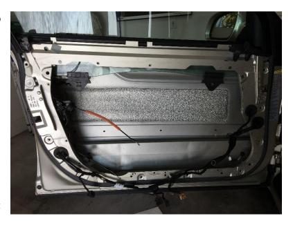
16. With the aluminum panel removed, you can see the door latch inside the door, and above that, the door handle. To make it easier to work on the handle, I lifted the window up as far as it would go (to the "window closed" position). Lift one side of the duct tape off the glass and pull the window up (with one hand on each side of the glass) until it is all the way up, and reattach the duct tape. Right, my window is now duct taped "fully up/closed."
