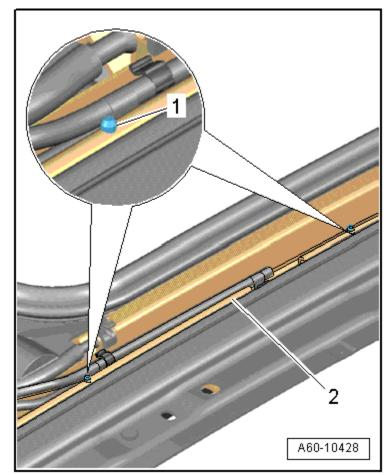
Remove the mount and cable forward in direction of -arrow-.
