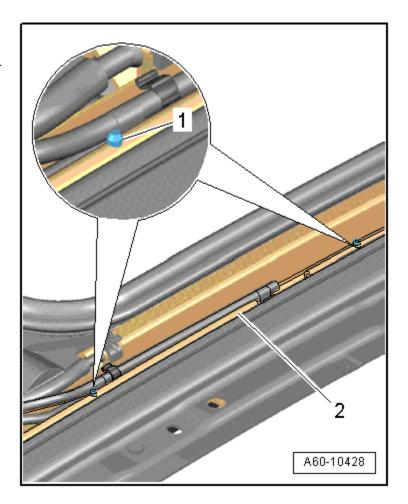
Remove the mount and the cable from the guide to the rear in direction of -arrow
