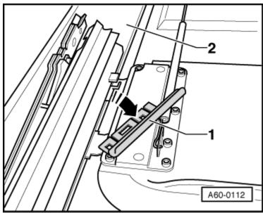
Slide inner trim -1- toward front and pull inward out of guide rail.
