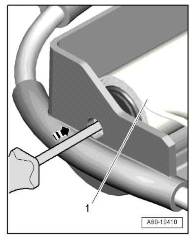
Lift the sunroof shade -1- upward at an angle on this side first...
