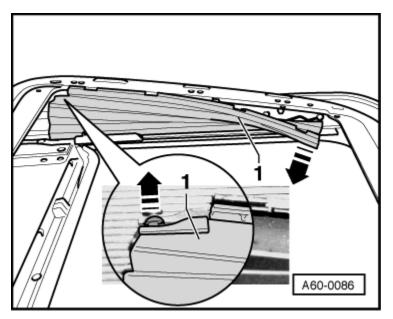
Pull off trim -1- from sunroof panel -1completely toward vehicle interior and fold it downward and away.
