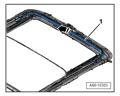
Press stops -2- for wind deflector toward rear under positioning bow -1- in direction of -arrow-.
