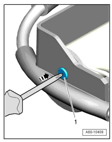
... and with the screwdriver push the axle on the sunroof shade -1- through the frame and hold it.
