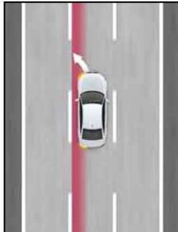
Audi active lane assist: Active steering torque when changing lane is suppressed if the indicator is active
