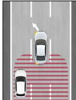
Audi side assist: Warns the driver if they begin to indicate when a vehicle is in a dangerous position.
