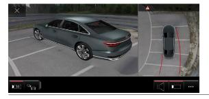
4 wide-angle environmental cameras cover the entire area directly around the vehicle and allow a variety of different views for even more comfortable maneuvering:
