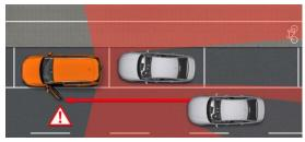
The exit warning warns of a possible collision with the rear approaching when the vehicle is opened Traffic. The system monitors the rear and side vehicle surroundings. Recognized from behind objects such as, for example, cars. When the door opening lever is pulled and a critical passenger other than the road user the warning strip in the door and the LED indicator on the side mirror on the affected side illuminate. At the same time, the door opening is briefly delayed.
